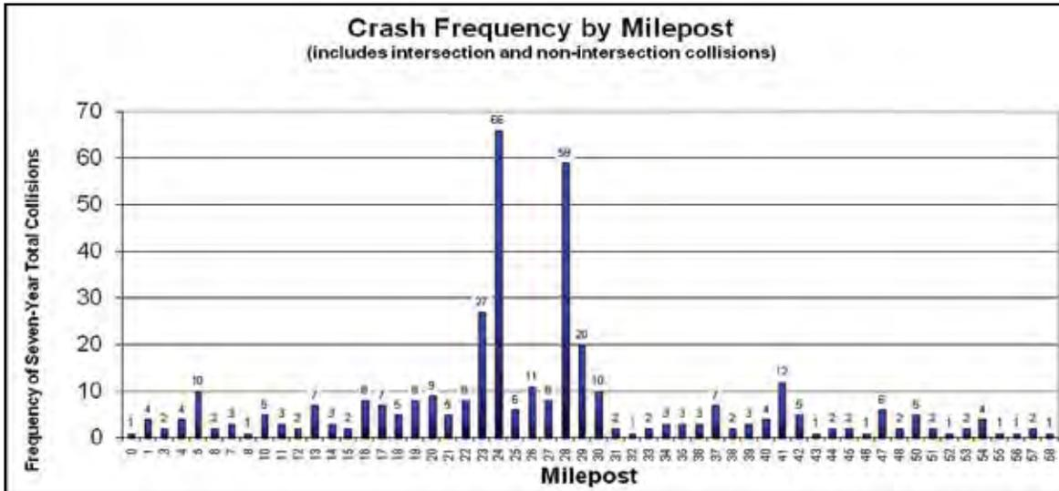
**NOTE:** Shows collision locations reported on N-12 over seven years (1999 through 2005). Distribution is shown in one-mile segments, so (for example) all collisions at MP 24.0 through 24.9 are shown at “MP24” in the chart.
