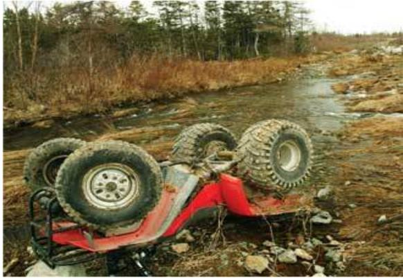
*Rollovers are the major mechanism for crashes of all-terrain vehicles (ATVs), alternatively called quad bikes (Quads). These crashes can occur on a clear day, when riding on flat ground or gentle slopes, and at relatively low speeds (less than 15 mph). One of the causes of severe injury and even death is being hit or pinned by the vehicle. Crush Protection Devices (CPDs) have been designed to protect riders from crush-related injuries in low speed rollovers to the side or to the rear.*
