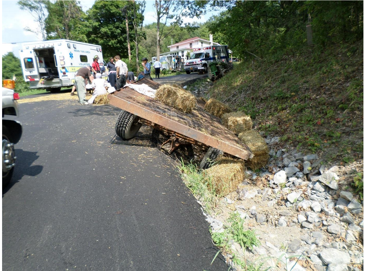
Yates County Mennonite farm tractor-wagon – 1 fatality and several injured. Steel lugs on new macadam – steep hill and overloaded wagon!
