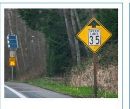
Photo: Courtesy of Neil Hetherington, WTI **Description:** Speed warning systems inform motorists that based on their vehicle speed, road geometry, weather conditions, or other factors, they are driving too fast. Some speed warning systems include:
