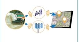
**Description:** Automatic vehicle location (AVL) systems track the real-time position of a vehicle. AVL uses a wireless communication system to communicate vehicle location to a central location or control center.
